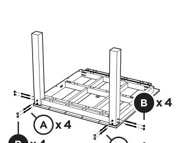
NOTE - Ensure thru holes in legs line up with pilot holes in aprons.
